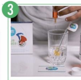
3 We need to take 100ml of tap water in a glass & Mix 4ml of color solvent with the help of a syringe.
